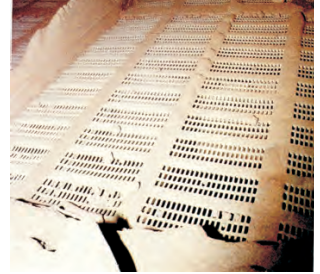
TIP TOP REMASCREEN stays almost completely clean thanks to its high selfcleaning effect.
